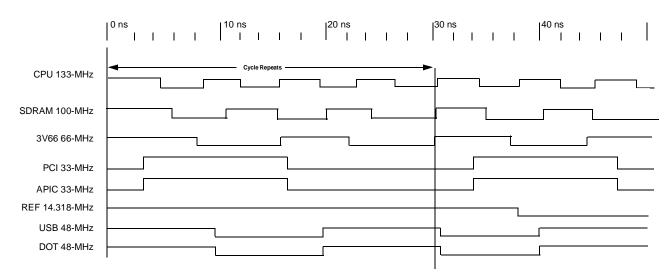
Figure 4. Group Offset Waveforms (133-MHz CPU/100-MHz SDRAM)
