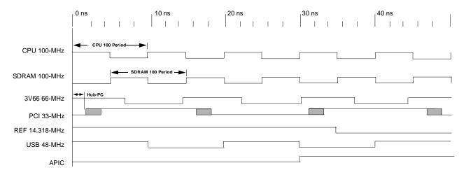
Figure 3. Group Offset Waveforms (100-MHz CPU Clock/100-MHz SDRAM Clock)
