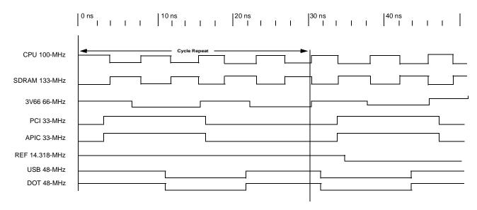
Figure 5. Group Offset Waveform (133-MHz CPU/133-MHz SDRAM)
