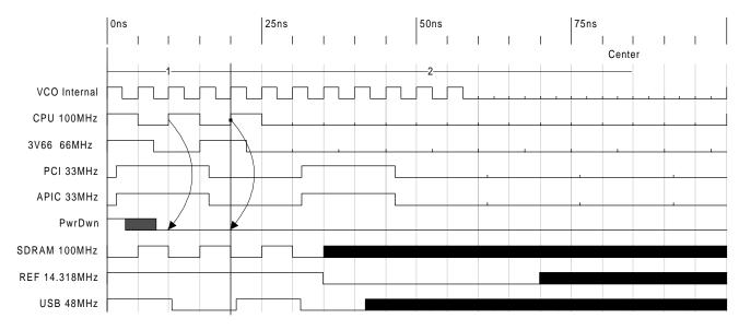
Figure 6. W229B PWRDWN# Timing Diagram<sup>[2, 3, 4, 5]</sup>
