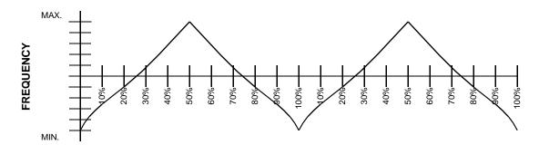
Figure 8. Typical Modulation Profile
